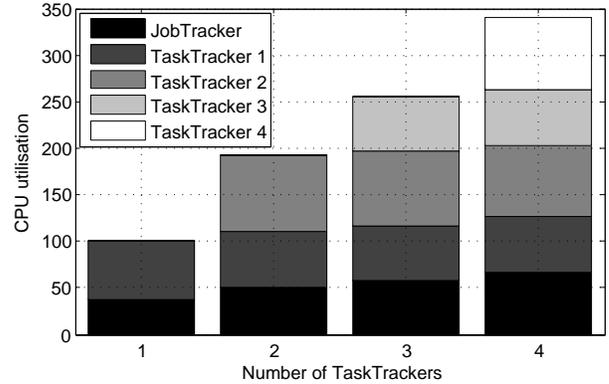
Fig. 5. CPU utilisation for window granularity.
