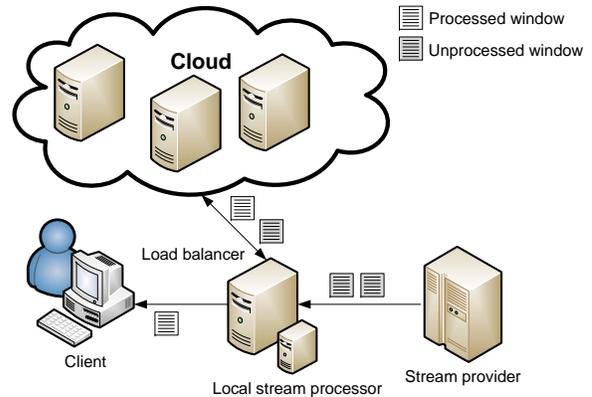
Fig. 1. Overview of combined stream processing system.
