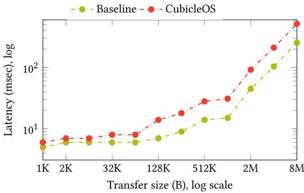
Figure 7: NGINX download latencies for different file sizes
