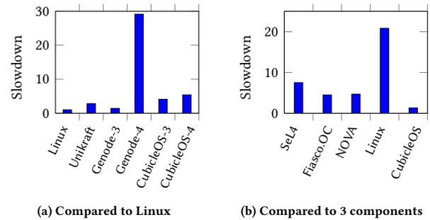
Figure 10: CubicleOS overhead compared to different kernels
