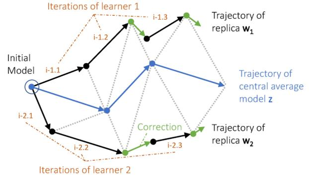
**Figure 2: Optimisation trajectories with independent model replicas under model averaging** (Two model replicas are trained independently with fixed batch sizes and corrected by an average model per iteration.)
