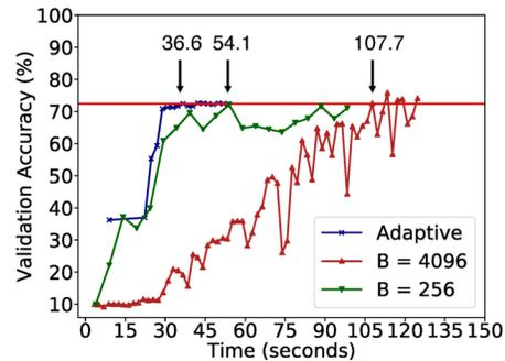
**Figure 5: Time-to-accuracy of adaptive and static batch size policies in KUNGFU** ( $B$  denotes batch size.)
