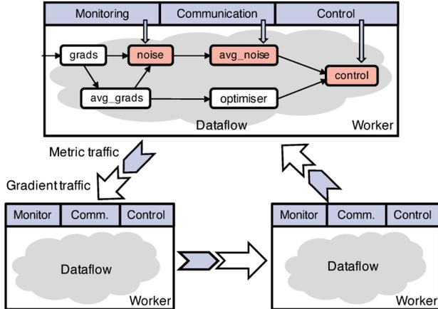
**Figure 4: Dynamic hyper-parameter management with three workers** (Each replicated training dataflow is augmented with monitoring and control operators. The monitored metrics are piggybacked as part of the communication for distributed gradient synchronisation.)
