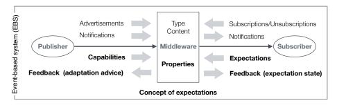
Fig. 1: Our concept extends the model of EBS (top) with capabilities, expectations and bidirectional feedback for runtime adaptation (bottom, bold).
